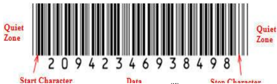
Figure 3. Structure of Barcode [15]
